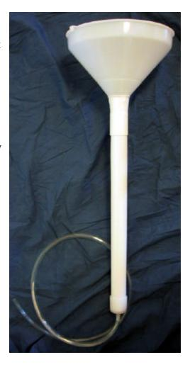
All carbon brands are poorly washed at the factory, so pour 3-5 litres of hot water through the activated carbon before you purify the spirit so as to wash out the salts not wanted in the spirit. Also the cleaning function of the carbon is enhanced if it is wet. Wait an hour or preferably 24 hours after washing and then wash again with 2 litres of hot water. Then you only have to pour the spirit in the top. Discard the water that comes out first.
