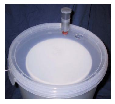
The immersion heater is bought in a pet shop. Normally used to heat a fish tank, and is available in various sizes and wattage.
