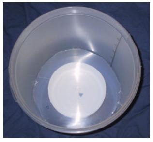
plate that is a perfect fit. Remember to place it high enough to give a tiny gap all around for the alcohol to run past.
