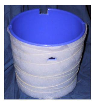
It is not difficult to insulate. Cut a strip of insulation making it 1 metre long and a bit wider than the vessel. (Roll out a length and cut off). Place it round the vessel and tie in place with cotton string. Cut off surplus insulation round the top and bottom of the vessel and cut out the holes. The insulation is very easy to cut so this is simple. Put on more layers and bind fast until you finally have a thickness of 10 mm or more. It's finished!
