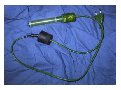
Unfortunately nearly all thermostats have a maximum setting of 32 degrees C. This heat is too low and it would take forever to produce anything. A suitable temperature range for this unit is 45-52 degrees C. Buy an immersion heater with a thermostat that goes up to 55 degrees C.
