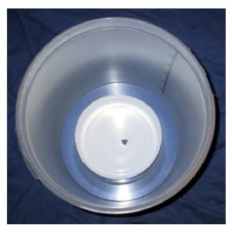
Make sure there is a hole in the item you intend to use so it does not float when alcohol runs down in the bottom of the 25-litre container. I have cut a little hole in the 10-litre vessel I am going to use as a support.
