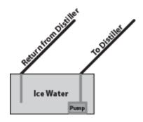
**Recirculated Water via Submersible Water Pump:** It is important that your water remains cool enough to condense the vapor efficiently. The simplest option is to use a large cooler with ice-water (or alternatively, cold water with frozen soda bottles). If necessary, add more ice as the distillation process warms the water. This dramatically reduces water consumption when compared with connecting to a water source. Setup as shown above.
