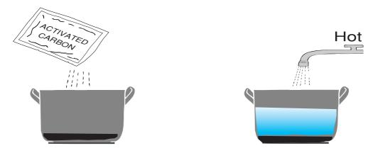
1. Pour the carbon into a stainless steel saucepan, and fill with at least twice as much boiling water.
