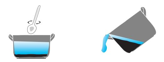
2. Stir with a large spoon, allow the carbon to sink to the bottom of the saucepan before discarding the surplus water. Repeat the process 4-5 times, making sure all soluble substances in the carbon have been washed out.
