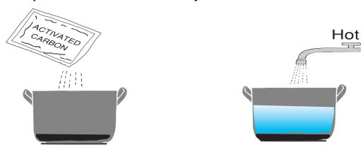
1. Pour the carbon into a stainless steel saucepan and add at least twice as much hot or boiling water.
